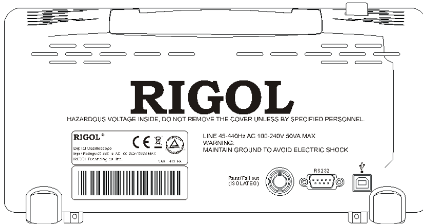
Figure 1- 3 Rear Panel Figure of DS1000E, DS1000D Series Oscilloscope
